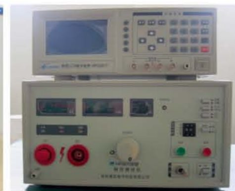
Digital electric bridge (Inductance testing)
