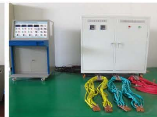
Strong current generator (Testing of temperature rise, range: 0-3000A)
